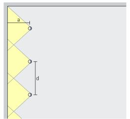
Accentuation Gimbal recessed spotlights accentuate artwork, products and architectural details effectively. The ideal angle of tilt ( $\alpha$ ) for this is around 30°. The object is modelled without distorting the effect as a result of excessive shadowing. It also prevents shadows cast by the observer.
