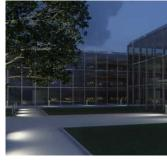
Different light distributions: wide or deep Floor washlights with a wide beam are ideal particularly for lighting pathways along walls and façades. Floor washlights with a deep beam are effective in illuminating open spaces such as squares or terraces.
