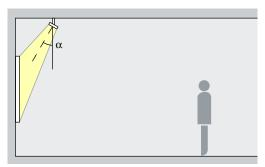
**Accentuation**Light Board spotlights accentuate artwork, products and architectural details effectively. The ideal angle of tilt ( $\alpha$ ) for this is around 30°. The object is modelled without distorting the effect as a result of excessive shadowing. It also prevents shadows cast by the observer.
