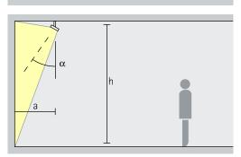
Wallwashing For uniform vertical illuminance, the distance (a) of Light Board lens wallwashers from the wall should be around one third of the room height (h). This results in an angle of tilt ( $\alpha$ ) of approx. 35°.
