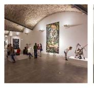
**Outstanding uniformity** To meet the stringent standards of ceiling washing, ERCO has developed luminaires that generate exceptionally uniform levels of illuminance.
