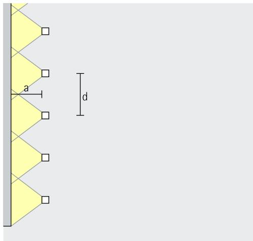
For good longitudinal uniformity, the spacing ( $d$ ) of Grasshopper lens wallwashers may be up to 1.2 times the offset from the wall ( $a$ ).
