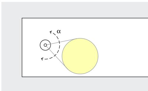
From a single position, the illuminated surface can be adjusted to the area of the visual task thanks to a luminaire head that can be rotated by 180° ( $\alpha$ ).
