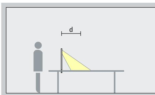
The position of Lucy task lights for desktop mounting depends on the surface to be illuminated. For optimum illumination of the desktop, the luminaire should be placed on the left side for right-handers and on the right for left-handers. The recommended mounting point is around 40-50cm (a) from the edge of the desk, with a distance (d) of around 50cm to the centre of the beam.
