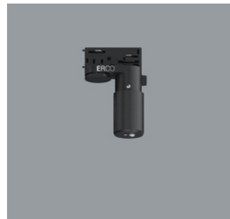
55249.000 ERCO Casambi motion detector with light sensor for ERCO 220-240V track. Setup via Casambi app (Android/iOS) with Bluetooth Low Energy (BLE)-capable mobile devices. Use for daylight-dependent light control with or without motion detector. Detection range of infrared (PIR) sensor 100°/ 5m. At 3m room height, this is a circle with diameter of approx. 7m. 3-phase adapter for ERCO 220-240V track: polymer, black. Black Weight 0.18kg CE UK
