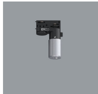
55250.000 ERCO Casambi motion detector with light sensor for ERCO 220-240V track. Setup via Casambi app (Android/iOS) with Bluetooth Low Energy (BLE)-capable mobile devices. Use for daylight-dependent light control with or without motion detector. Detection range of infrared (PIR) sensor 100°/ 5m. At 3m room height, this is a circle with diameter of approx. 7m. 3-phase adapter for ERCO 220-240V track: polymer, black. Silver Weight 0.18kg CE UK
