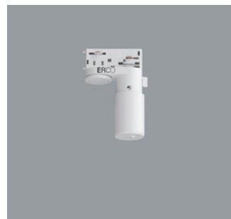
55248.000 ERCO Casambi motion detector with light sensor for ERCO 220-240V track. Setup via Casambi app (Android/iOS) with Bluetooth Low Energy (BLE)-capable mobile devices. Use for daylight-dependent light control with or without motion detector. Detection range of infrared (PIR) sensor 100°/ 5m. At 3m room height, this is a circle with diameter of approx. 7m. 3-phase adapter for ERCO 220-240V track: plastic, white. White Weight 0.18kg CE UK
