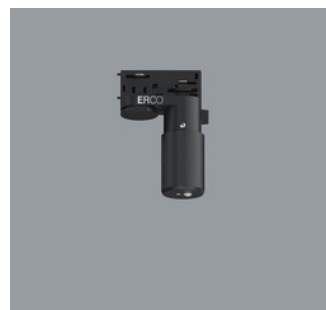
55249.000 ERCO Casambi motion detector with light sensor for ERCO 220-240V track. Setup via Casambi app (Android/iOS) with Bluetooth Low Energy (BLE)-capable mobile devices. Use for daylight-dependent light control with or without motion detector. Detection range of infrared (PIR) sensor 100°/ 5m. At 3m room height, this is a circle with diameter of approx. 7m. 3-phase adapter for ERCO 220-240V track: polymer, black.
