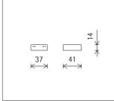
ERCO Casambi motion detector with light sensor for ERCO 220-240V track. Setup via Casambi app (Android/iOS) with Bluetooth Low Energy (BLE)capable mobile devices. Use for daylight-dependent light control with or without motion detector. Detection range of infrared (PIR) sensor 100°/5m. At 3m room height, this is a circle with diameter of approx. 7m. 3-phase adapter for ERCO 220-240V track: polymer, black.
