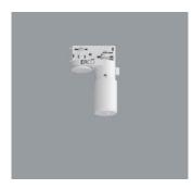
ERCO Casambi motion detector with light sensor for ERCO 220-240V track. Setup via Casambi app (Android/iOS) with Bluetooth Low Energy (BLE)capable mobile devices. Use for daylight-dependent light control with or without motion detector. Detection range of infrared (PIR) sensor 100°/5m. At 3m room height, this is a circle with diameter of approx. 7m. 3-phase adapter for ERCO 220-240V track: plastic, white.
