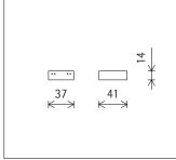
ERCO Casambi motion detector with light sensor for ERCO 220-240V track. Setup via Casambi app (Android/iOS) with Bluetooth Low Energy (BLE)capable mobile devices. Use for daylight-dependent light control with or without motion detector. Detection range of infrared (PIR) sensor 100°/ 5m. At 3m room height, this is a circle with diameter of approx. 7m.
