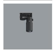
ERCO Casambi motion detector with light sensor for ERCO 220-240V track. Setup via Casambi app (Android/iOS) with Bluetooth Low Energy (BLE)capable mobile devices. Use for daylight-dependent light control with or without motion detector. Detection range of infrared (PIR) sensor 100°/5m. At 3m room height, this is a circle with diameter of approx. 7m. 3-phase adapter for ERCO 220-240V track: polymer, black.
