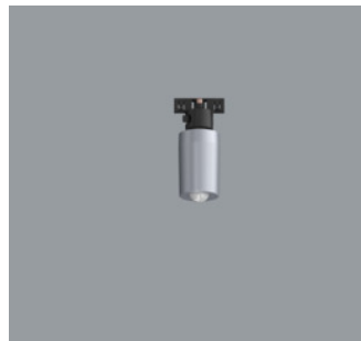
56013.000 ERCO Casambi motion detector with light sensor for ERCO Minirail 48V track. Setup via Casambi app (Android/iOS) with Bluetooth Low Energy (BLE)-capable mobile devices. Use for daylight-dependent light control with or without motion detector. Detection range of infrared (PIR) sensor 100°/ 5m. At 3m room height, this is a circle with diameter of approx. 7m. Minirail adapter for ERCO Minirail 48V track: polymer, black. Available from 2nd quarter 2023 Silver Weight 0.18kg CE
