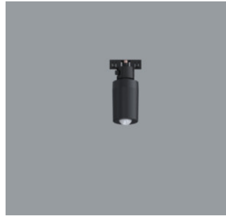
56012.000 ERCO Casambi motion detector with light sensor for ERCO Minirail 48V track. Setup via Casambi app (Android/iOS) with Bluetooth Low Energy (BLE)-capable mobile devices. Use for daylight-dependent light control with or without motion detector. Detection range of infrared (PIR) sensor 100°/ 5m. At 3m room height, this is a circle with diameter of approx. 7m. Minirail adapter for ERCO Minirail 48V track: polymer, black. Available from 2nd quarter 2023 Black Weight 0.18kg CE
