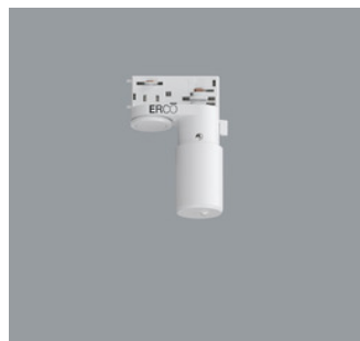
55248.000 ERCO Casambi motion detector with light sensor for ERCO 220-240V track. Setup via Casambi app (Android/iOS) with Bluetooth Low Energy (BLE)-capable mobile devices. Use for daylight-dependent light control with or without motion detector. Detection range of infrared (PIR) sensor 100°/ 5m. At 3m room height, this is a circle with diameter of approx. 7m. 3-phase adapter for ERCO 220-240V track: plastic, white. White Weight 0.18kg CE, RoHS, WEEE, REACH, PSE, UKCA
