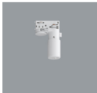
55248.000 ERCO Casambi motion detector with light sensor for ERCO 220-240V track. Setup via Casambi app (Android/iOS) with Bluetooth Low Energy (BLE)-capable mobile devices. Use for daylight-dependent light control with or without motion detector. Detection range of infrared (PIR) sensor 100°/ 5m. At 3m room height, this is a circle with diameter of approx. 7m. 3-phase adapter for ERCO 220-240V track: plastic, white. White Weight 0.18kg CE, RoHS, WEEE, REACH, EN60598-1, EN60598-2-1, EN60598-2-2, EN60598-2-3, EN60598-2-4, EN60598-2-5, EN60598-2-6, EN60598-2-7, EN60598-2-8, EN60598-2-9, EN60598-2-10, EN60598-2-11, EN60598-2-12, EN60598-2-13, EN60598-2-14, EN60598-2-15, EN60598-2-16, EN60598-2-17, EN60598-2-18, EN60598-2-19, EN60598-2-20, EN60598-2-21, EN60598-2-22, EN60598-2-23, EN60598-2-24, EN60598-2-25, EN60598-2-26, EN60598-2-27, EN60598-2-28, EN60598-2-29, EN60598-2-30, EN60598-2-31, EN60598-2-32, EN60598-2-33, EN60598-2-34, EN60598-2-35, EN60598-2-36, EN60598-2-37, EN60598-2-38, EN60598-2-39, EN60598-2-40, EN60598-2-41, EN60598-2-42, EN60598-2-43, EN60598-2-44, EN60598-2-45, EN60598-2-46, EN60598-2-47, EN60598-2-48, EN60598-2-49, EN60598-2-50, EN60598-2-51, EN60598-2-52, EN60598-2-53, EN60598-2-54, EN60598-2-55, EN60598-2-56, EN60598-2-57, EN60598-2-58, EN60598-2-59, EN60598-2-60, EN60598-2-61, EN60598-2-62, EN60598-2-63, EN60598-2-64, EN60598-2-65, EN60598-2-66, EN60598-2-67, EN60598-2-68, EN60598-2-69, EN60598-2-70, EN60598-2-71, EN60598-2-72, EN60598-2-73, EN60598-2-74, EN60598-2-75, EN60598-2-76, EN60598-2-77, EN60598-2-78, EN60598-2-79, EN60598-2-80, EN60598-2-81, EN60598-2-82, EN60598-2-83, EN60598-2-84, EN60598-2-85, EN60598-2-86, EN60598-2-87, EN60598-2-88, EN60598-2-89, EN60598-2-90, EN60598-2-91, EN60598-2-92, EN60598-2-93, EN60598-2-94, EN60598-2-95, EN60598-2-96, EN60598-2-97, EN60598-2-98, EN60598-2-99, EN60598-2-100
