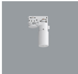
55248.000 ERCO Casambi motion detector with light sensor for ERCO 220-240V track. Setup via Casambi app (Android/iOS) with Bluetooth Low Energy (BLE)-capable mobile devices. Use for daylight-dependent light control with or without motion detector. Detection range of infrared (PIR) sensor 100°/ 5m. At 3m room height, this is a circle with diameter of approx. 7m. 3-phase adapter for ERCO 220-240V track: plastic, white. White Weight 0.18kg
