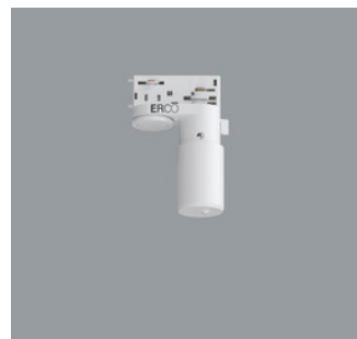
55248.000 ERCO Casambi motion detector with light sensor for ERCO 220-240V track. Setup via Casambi app (Android/iOS) with Bluetooth Low Energy (BLE)-capable mobile devices. Use for daylight-dependent light control with or without motion detector. Detection range of infrared (PIR) sensor 100°/ 5m. At 3m room height, this is a circle with diameter of approx. 7m. 3-phase adapter for ERCO 220-240V track: plastic, white. White Weight 0.18kg CE, RoHS, REACH, WEEE, PSE, UKCA
