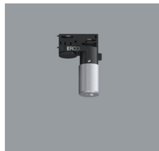
55250.000 ERCO Casambi motion detector with light sensor for ERCO 220-240V track. Setup via Casambi app (Android/iOS) with Bluetooth Low Energy (BLE)-capable mobile devices. Use for daylight-dependent light control with or without motion detector. Detection range of infrared (PIR) sensor 100°/ 5m. At 3m room height, this is a circle with diameter of approx. 7m. 3-phase adapter for ERCO 220-240V track: polymer, black. Silver Weight 0.18kg CE, RoHS, WEEE, REACH, EN60598-1, EN60598-2-1
