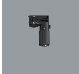
55249.000 ERCO Casambi motion detector with light sensor for ERCO 220-240V track. Setup via Casambi app (Android/iOS) with Bluetooth Low Energy (BLE)-capable mobile devices. Use for daylight-dependent light control with or without motion detector. Detection range of infrared (PIR) sensor 100°/ 5m. At 3m room height, this is a circle with diameter of approx. 7m. 3-phase adapter for ERCO 220-240V track: polymer, black. Black Weight 0.18kg CE, RoHS, WEEE, REACH, EN60598-1, EN60598-2-1
