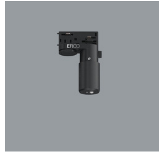
55249.000 ERCO Casambi motion detector with light sensor for ERCO 220-240V track. Setup via Casambi app (Android/iOS) with Bluetooth Low Energy (BLE)-capable mobile devices. Use for daylight-dependent light control with or without motion detector. Detection range of infrared (PIR) sensor 100°/ 5m. At 3m room height, this is a circle with diameter of approx. 7m. 3-phase adapter for ERCO 220-240V track: polymer, black. Black Weight 0.18kg CE, RoHS, WEEE, REACH, PSE, UKCA
