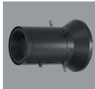
AC002164 Lens unit extra wide flood Polymer, black, rotatable through 360°. Replacement without tools. Spherolit lens made of optical polymer.
