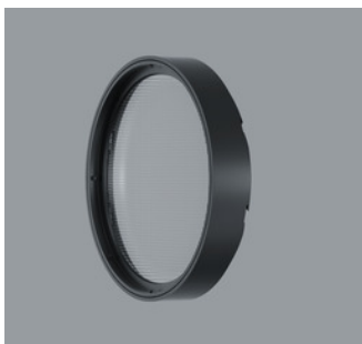
AC002165 Lens unit oval flood Polymer, black, rotatable through 360°. Replacement without tools. Anti-reflective Spherolit lens made of optical polymer.
