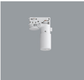
55248.000 ERCO Casambi motion detector with light sensor for ERCO 220-240V track. Setup via Casambi app (Android/iOS) with Bluetooth Low Energy (BLE)-capable mobile devices. Use for daylight-dependent light control with or without motion detector. Detection range of infrared (PIR) sensor 100°/ 5m. At 3m room height, this is a circle with diameter of approx. 7m. 3-phase adapter for ERCO 220-240V track: plastic, white. White Weight 0.18kg CE
