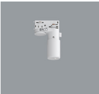
55248.000 ERCO Casambi motion detector with light sensor for ERCO 220-240V track. Setup via Casambi app (Android/iOS) with Bluetooth Low Energy (BLE)-capable mobile devices. Use for daylight-dependent light control with or without motion detector. Detection range of infrared (PIR) sensor 100°/ 5m. At 3m room height, this is a circle with diameter of approx. 7m. 3-phase adapter for ERCO 220-240V track: plastic, white.
