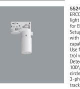
55248.000 ERCO Casambi motion detector with light sensor for ERCO 220-240V track. Setup via Casambi app (Android/iOS) with Bluetooth Low Energy (BLE)capable mobile devices. Use for daylight-dependent light control with or without motion detector. Detection range of infrared (PIR) sensor 100°/5m. At 3m room height, this is a circle with diameter of approx. 7m. 3-phase adapter for ERCO 220-240V track: plastic, white. White
