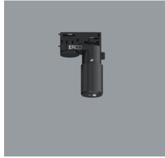
55249.000 ERCO Casambi motion detector with light sensor for ERCO 220-240V track. Setup via Casambi app (Android/iOS) with Bluetooth Low Energy (BLE)-capable mobile devices. Use for daylight-dependent light control with or without motion detector. Detection range of infrared (PIR) sensor 100°/ 5m. At 3m room height, this is a circle with diameter of approx. 7m. 3-phase adapter for ERCO 220-240V track: polymer, black. Black Weight 0.18kg CE
