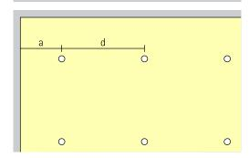
The recommended offset from the wall is half the luminaire spacing.
