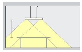
**General lighting**To achieve a high level of uniformity and good facial recognition when illuminating single workstations, Jilly pendant luminaires with extra wide flood light distribution should be suspended at a height (h) of approx. 1.2m above the desk plane.
