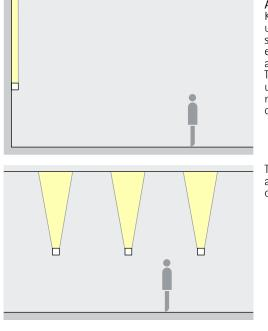
Accentuation Kubus façade luminaires with upward and downward beam emisupward and downward beam emis-sion structure large façades, whilst emphasising the three-dimension-ality of materials with grazing light. To avoid glare, luminaires with an upward light emission are best mounted above eye-level of the obscarver. observer.
