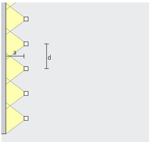
For good longitudinal uniformity, the spacing ( $d$ ) of Lightscan lens wallwashers may be up to 1.2 times the offset from the wall ( $a$ ).
