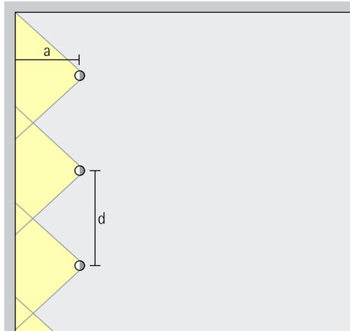
For good longitudinal uniformity, the spacing (d) of Quintessence lens wallwashers may be up to 1.3 times the offset from the wall (a).
