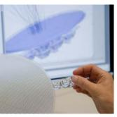
More light on the target surface The lens system, developed and manufactured in-house, precisely projects the light with no spill light. The accent lighting of the ERCO spotlight thus sets itself clearly apart from conventional spotlights.
