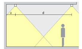
The wall offset should be half the luminaire spacing.
