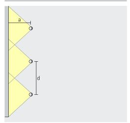
For good longitudinal uniformity, the distance (d) of Iku lens wall-washers may be up to 1.3 times the distance to the wall (a).
