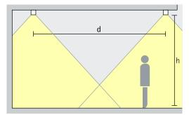
**General lighting**For uniform ambient lighting, the approximate distance (d) between two lku downlights may be up to 1.5 times the height (h) of the luminaire above the working plane.
