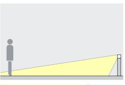
Kubus bollard luminaires with deep beam light distribution directed forward provide subtle light for a glare-free and uniform illumination of open areas.
