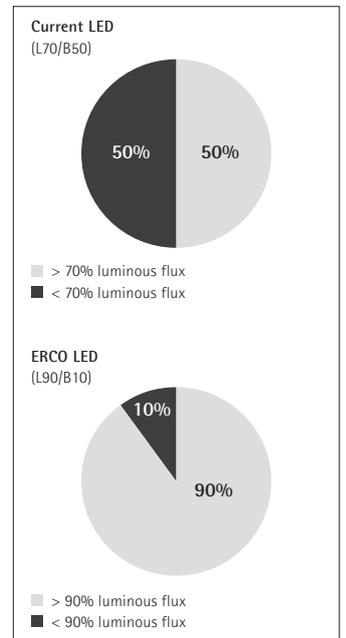
Comparing the reduction in luminous flux of a standard LED with an ERCO high-power LED after 50,000 operating hours illustrates the superior efficiency of ERCO LEDs.
