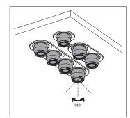
The stem-mounted luminaire consists of the stem and at least one light head. The luminaire is suitable for floor or ceiling mounting in a showcase. The stem is height-adjustable. The light head is attached by magnets at the end of the stem and at the light head. You can mount the light head in one direction only because of the polarity of the magnets.
